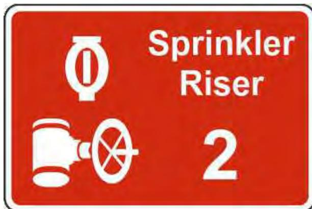
Building Systems Identification Sign. Many problems that the fire department are called for are due to a buildings mechanical, electrical, or other type of systems. In order to investigate the cause of the problem, firefighters must be able to locate them quickly. This includes, but it not limited to: elevator control room, electrical room, HVAC, hot water heaters, boilers, and more. The specification of these signs are as follows:
